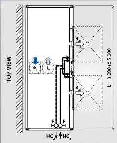
The diameter of the connecting pipe is 1", the pipe up to the ball valve is supplied by ATREA.
