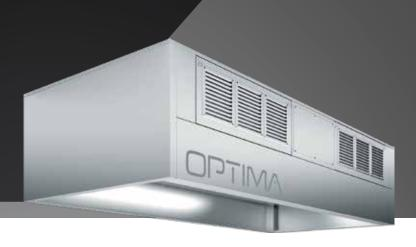
**Kitchen hoods OPTIMA with heat recovery efficiency up to 75** % efficiently extract and filter waste air, at the same time conveniently supplying re-heated fresh air to kitchens of all sizes and configurations, with automatic operation. Compared with the standard range they additionally include **integrated electrical reheaters or water-to-air heat exchangers** to heat or cool supply air.
