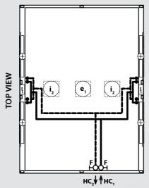
The diameter of the connecting pipe is 1", the pipe up to the ball valve is supplied by ATREA.
