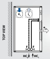
The diameter of the connecting pipe is 1", the pipe up to the ball valve is supplied by ATREA.
